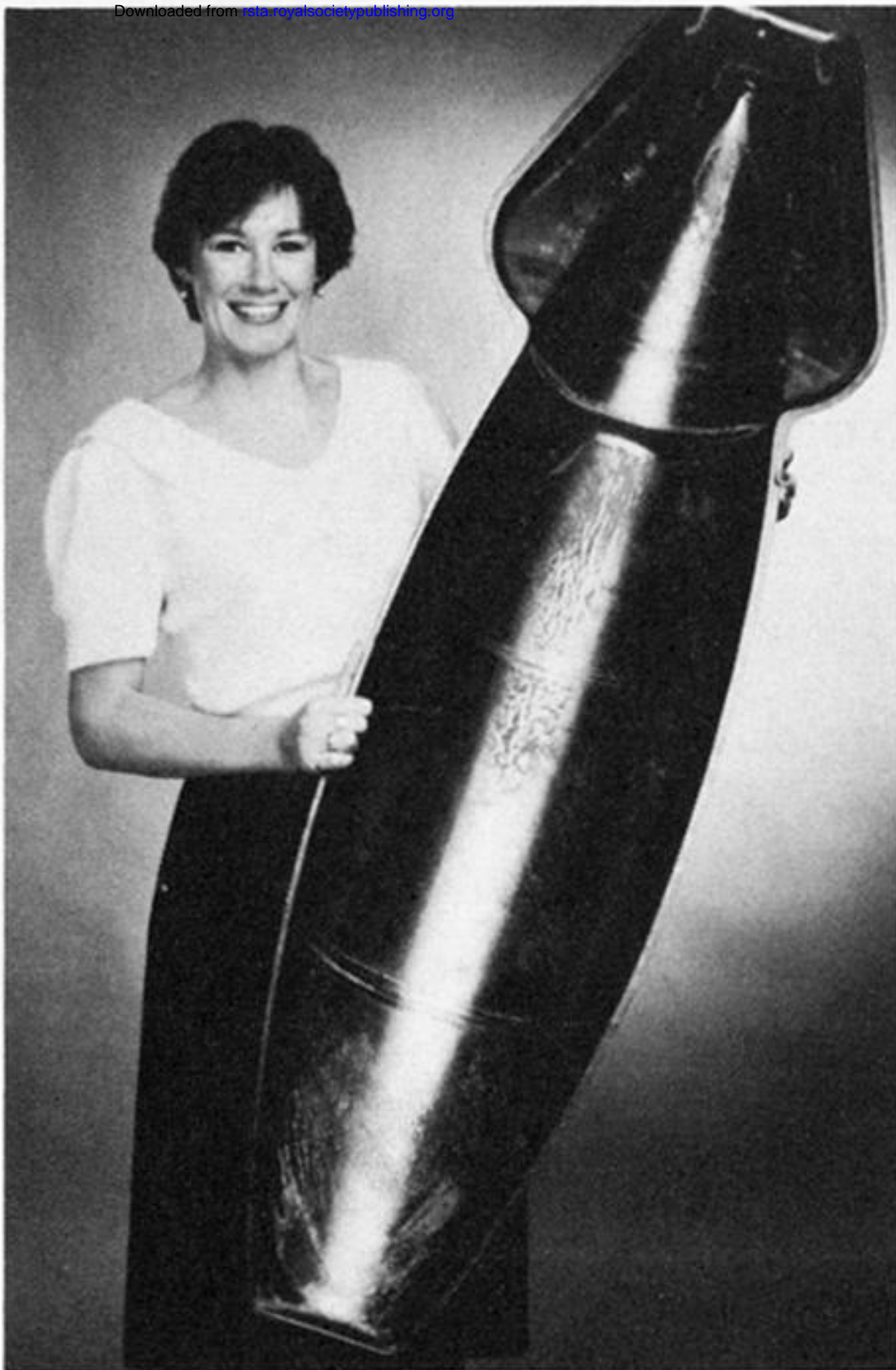
FIGURE 9. Superplastic diaphragm formed component.
