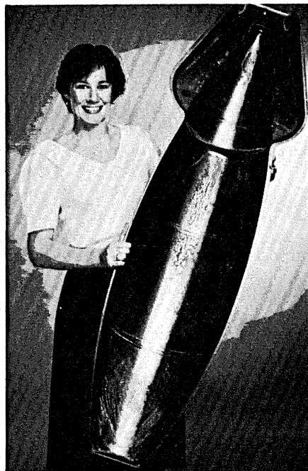
FIGURE 9. Superplastic diaphragm formed component.
